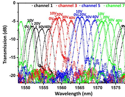
Fig. 7. Transmission of output channel 1, 3, 5 and 7 of the AWG under 0 W, 10 V (0.08 W), 20 V (0.32 W), 30 V (0.72 W), and 40 V (1.26 W).
