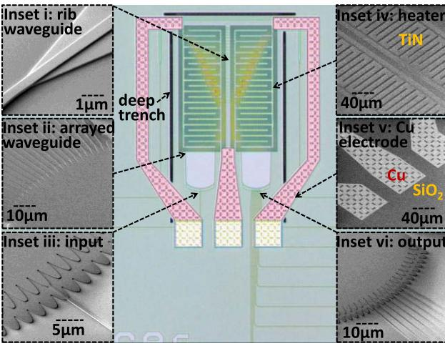
Fig. 4. Microscope image of the tunable silicon AWG. Inset i: SEM image of the rib waveguide. Inset ii: SEM image of the arrayed waveguide. Inset iii: SEM image of the input waveguide. Inset iv: SEM image of the TiN heater. Inset v: SEM image of the Cu electrode. Inset vi: SEM image of 8 channels output.
