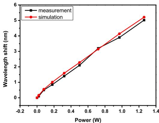
Fig. 8. Measured and simulated wavelength shift under different bias powers.
