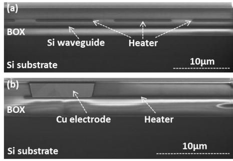
Fig. 5. Cross-sectional SEM images of (a) the heater and the Si waveguide; (b) the Cu electrode and vias to heater.
