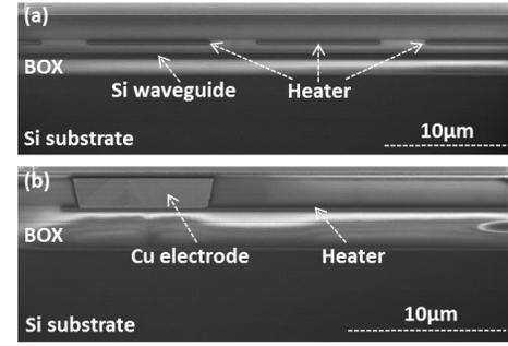
Fig. 5. Cross-sectional SEM images of (a) the heater and the Si waveguide; (b) the Cu electrode and vias to heater.
