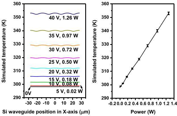
Fig. 3. Simulated temperature distribution of the silicon waveguide under different bias voltages/powers on TiN heater. Less than 1 K temperature variation is observed from the error bar.
