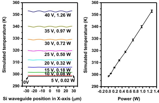
Fig. 3. Simulated temperature distribution of the silicon waveguide under different bias voltages/powers on TiN heater. Less than 1 K temperature variation is observed from the error bar.
