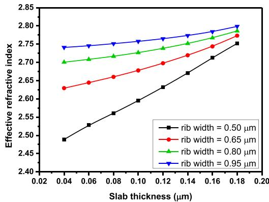
Fig. 1. Simulated effective-refractive-index ( $n_{eff}$ ) of the ridge waveguide with the different slab thicknesses and rib widths.
