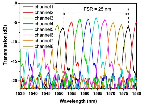
Fig. 6. Transmission of 8 channels output before heating.
