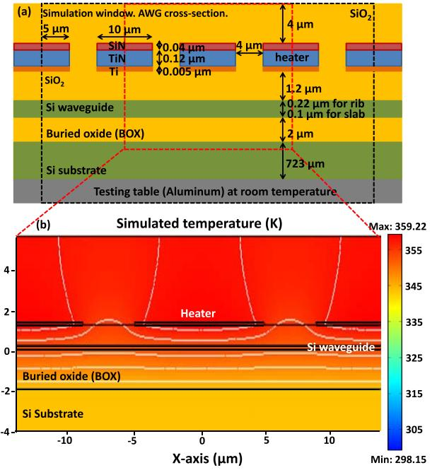
Fig. 2. (a) Thermal simulation structure (not to scale). (b) Simulated cross-sectional thermal distribution when a 40V bias voltage (1.26 W power) is applied to the TiN heater. The temperature of the silicon waveguide is  $\sim$ 53K higher than the room temperature (298.15 K). The white line in the figure is the isothermal line. The simulation image is partially presented.
