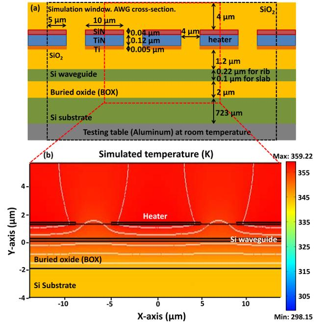
Fig. 2. (a) Thermal simulation structure (not to scale). (b) Simulated cross-sectional thermal distribution when a 40V bias voltage (1.26 W power) is applied to the TiN heater. The temperature of the silicon waveguide is  $\sim 53\text{K}$  higher than the room temperature (298.15 K). The white line in the figure is the isothermal line. The simulation image is partially presented.
