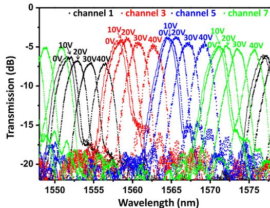
Fig. 7. Transmission of output channel 1, 3, 5 and 7 of the AWG under 0 V (0 W), 10 V (0.08 W), 20 V (0.32 W), 30 V (0.72 W), and 40 V (1.26 W).
