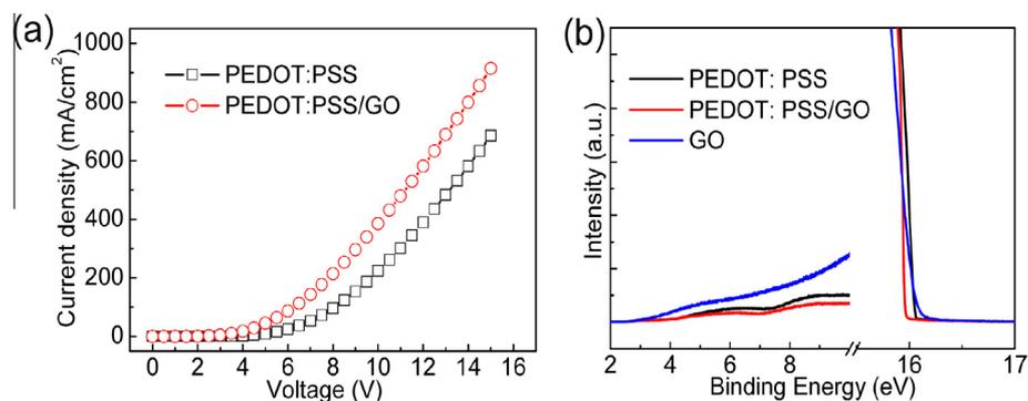
**Fig. 3.** (a) Current density–voltage characteristics of hole-only devices with PEDOT:PSS anode and PEDOT:PSS/GO (15:1) composite anode. (b) UPS spectra of PEDOT:PSS, PEDOT:PSS/GO (15:1) and GO films.
