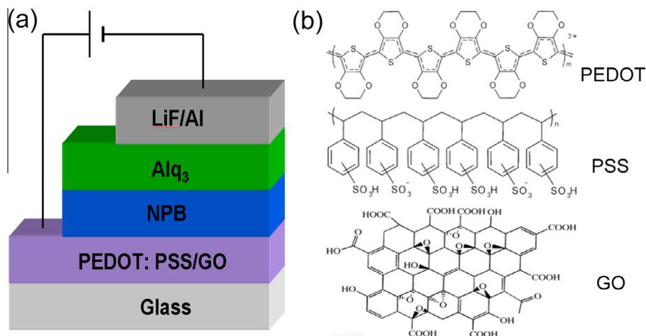
Fig. 1. (a) Schematic structure of OLEDs based on the PEDOT:PSS/GO composite anode. (b) The chemical structures of the PEDOT:PSS and GO.
