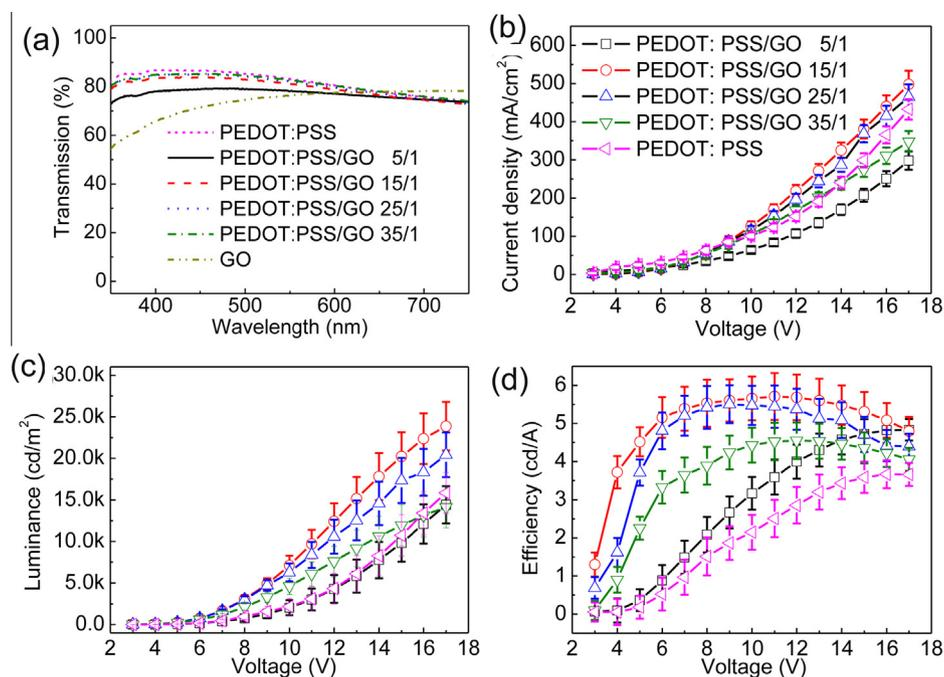
Fig. 2. (a) Transmittance spectra of the pure PEDOT:PSS film and PEDOT:PSS/GO composite films with different doping ratio. (b) Current density–voltage, (c) luminance–voltage and (d) efficiency–voltage characteristics of the OLEDs with composite anodes in different doping ratio.
