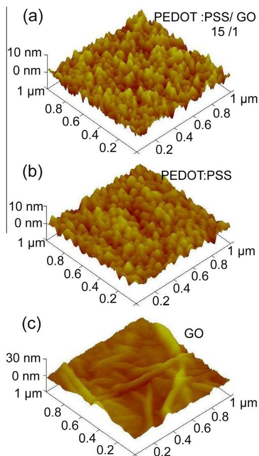
**Fig. 4.** Surface morphologies of the PEDOT:PSS/GO (15/1) films (a), PEDOT:PSS films (b) and GO films (c).
