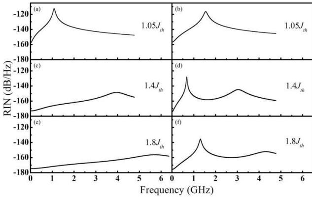
Fig. 6. Comparison of the RIN spectra for a hybrid laser (a) (c) (e) and diode laser (b) (d) (f) with same ridge width of  $4\mu\text{m}$ , under different injection current densities: Injection current density is  $1.05J_{th}$  (first row); Injection current density is  $1.4J_{th}$  (second row); Injection current density is  $1.8J_{th}$  (third row).
