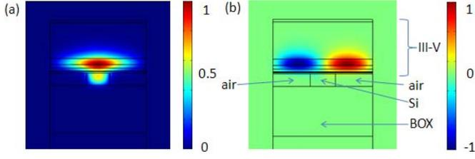
Fig. 1. The optical field distributions of the TE<sub>00</sub> (a) and TE<sub>10</sub> (b) mode of a hybrid laser with a 4  $\mu\text{m}$ -wide III-V ridge, a 1  $\mu\text{m}$ -wide and 500 nm-high Si ridge with arrows indicating the silicon-on-insulator (SOI) structure. BOX in (b) refers to buried oxide.
