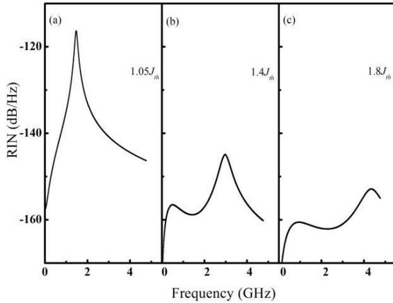
Fig. 3. The RIN spectra for hybrid laser with a  $3\mu\text{m}$  III-V ridge width, 220 nm Si ridge height under different injection current density: (a) Injection current density is  $1.05J_{th}$ ; (b) Injection current density is  $1.4J_{th}$ ; (c) Injection current density is  $1.8J_{th}$ .
