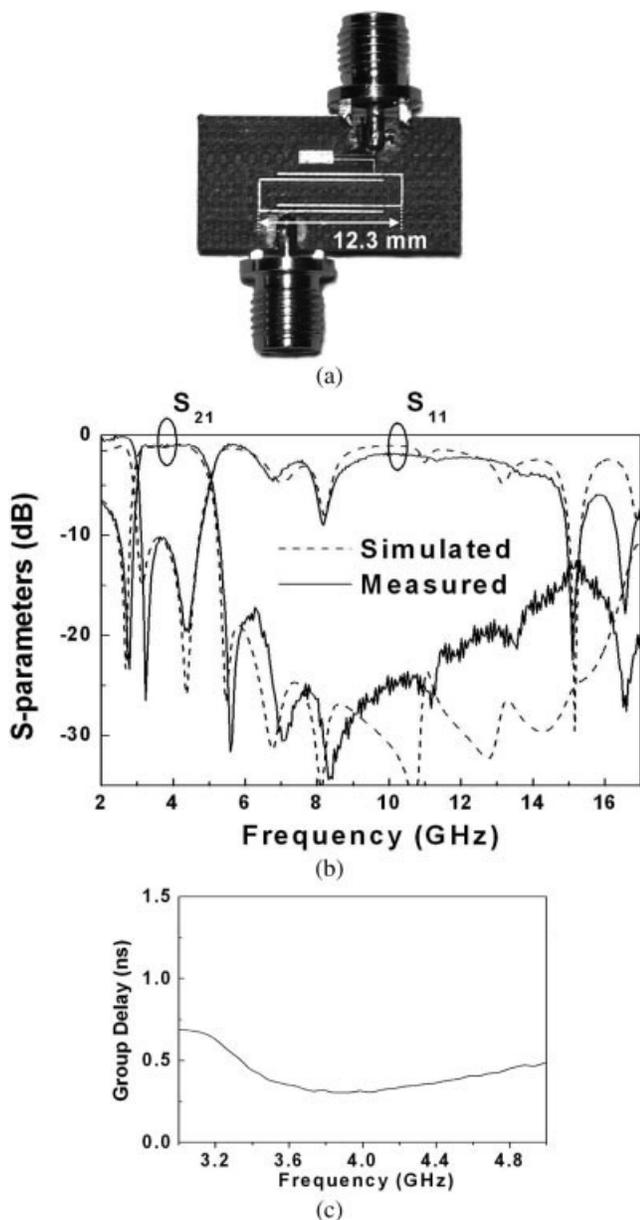
**Figure 5** (a) Picture, (b) simulated and measured frequency response, and (c) group delay of the fabricated BPF with the MTZS
