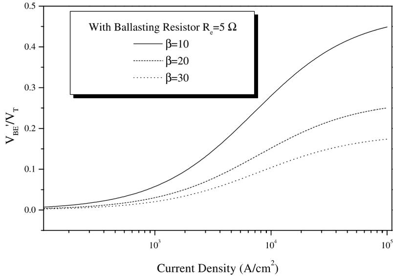
Fig. 2. Ratio of  $V_{BE}'$  and  $V_T$  as function of average emitter current density for various values of current gain with ballasting resistor.
