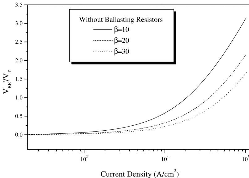
Fig. 1. Ratio of  $V_{BE}'/V_T$  and  $V_T$  as function of average emitter current density for various values of current gain without ballasting resistor.
