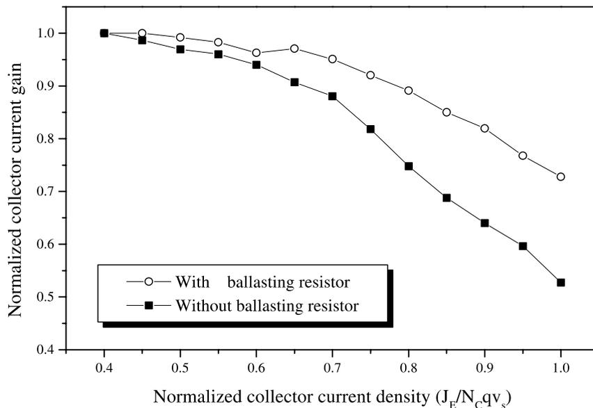
Fig. 4. Measured current gains vs.  $J_E$ .
