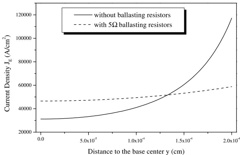
Fig. 3.  $J_E(y)$  vs. distance from emitter center with and without ballasting resistor  $R_c$ .
